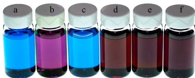
Figure 6. Effect of anions (as (C_4H_9)_4 N^+ salt) on color changes of 2 in DMSO/H 2 O (80:20 v/v) ( 5 \times 10^{-5} M) after the addition of 2 equiv of anion: (a) 2 only; (b) 2 +maleate; (c) 2 +fumarate; (d) 2 +phthalate; (e) 2 +isophthalate and (f) 2 +terephthalate.
